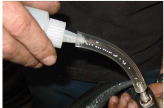
4. Install the valve core and air up tires. When checking pressure and airing up tires make sure the valve stems are on the bottom of the tire, or nearly so.
