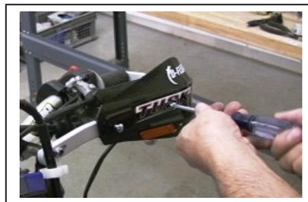
9. Making sure the wire paths are clean and won't interfere with anything, go ahead and plug in horn, signals, relay, on/off switch, and control switch to the wiring harness. (refer to wiring diagram that came with the harness)
