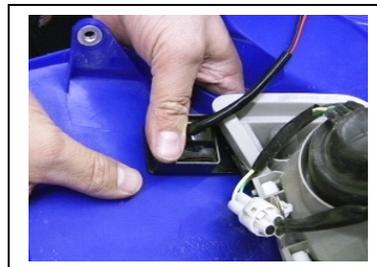
8. Install front turn signals. If you are using the "mini stalk" turn signals, they can be installed by drilling mounting holes to the plastic headlight housing. The "handguard" signals can be installed to the handlebars with the included mounts, or can be installed directly to aluminum wrap-around style handguards (Tusk part # 1096330001 – sold separately).
