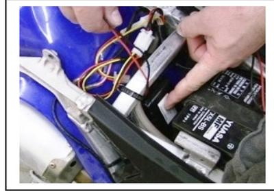
11. Double check the wiring by referring to harness wiring diagram. Plug the battery into the harness and test the kit. Turn the On/Off switch to the "On" position. The tail light should be on. Test the turn signals, horn, and brake to make sure everything is functioning. If there are problems, double check all wiring and 5 amp fuse.
