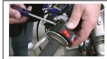
7. Install the horn and flasher relay. These can be installed in multiple locations on the front of the machine. Choose a location most suitable for your application. The mounting hole can be drilled larger if needed. Velcro with an adhesive back (not included) may be used on the flasher relay if desired.
