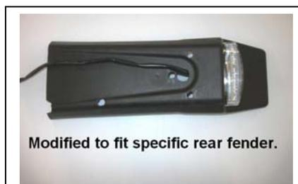
3. Align flush mount turn signals in desired location. Drill holes for the turn signal wires. Run the wires up through the tail/brake light unit (same wire path as tail/brake light wires) to keep them protected. Make sure the desired turn signal location is clean by wiping the area with rubbing alcohol or contact cleaner. Adhere the turn signal.
