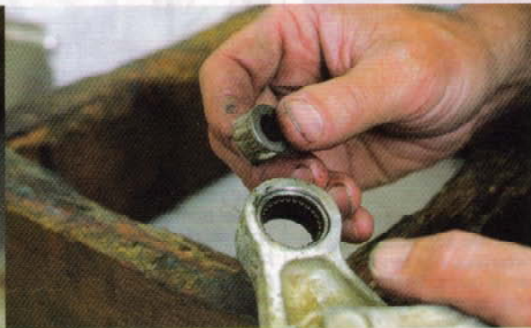
5 Putting the bearing in the freezer for about an hour helps to contract the metal and make it slide into the linkage knuckle easier.
