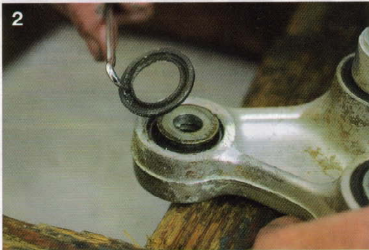
2 With the help of a sharp implement, remove the seal. Don't hurt yourself.
