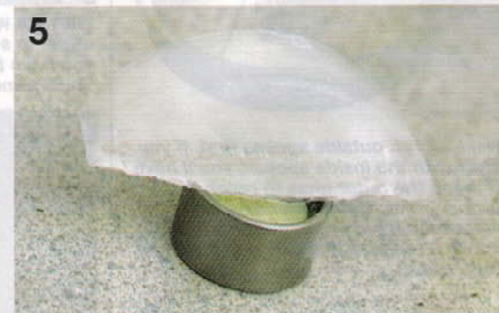
5 Putting the bearing in the freezer for about an hour helps to contract the metal and make it slide into the linkage knuckle easier.
