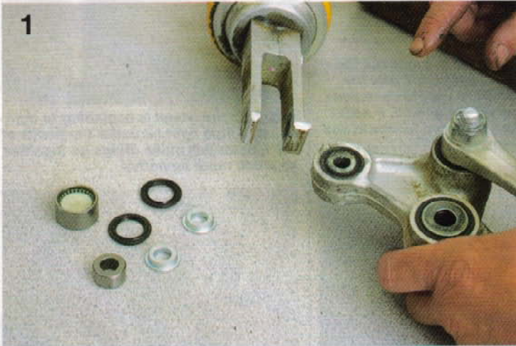
1 The goods to replace the lower shock mount bearing from Pivot Works.
