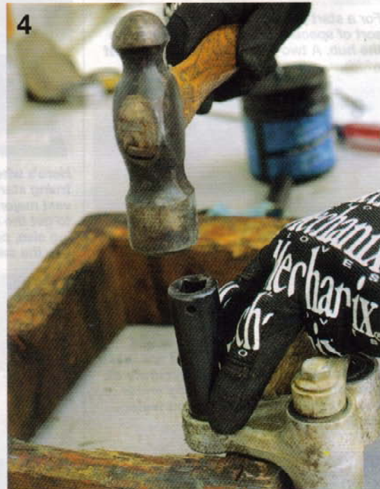
4 Find a socket that is the same size as the bearing and carefully hammer it out. Support the knuckle on wood. If it's hard to get out you can use a vise to get it started.
