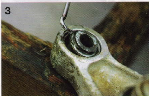
2 With the help of a sharp implement, remove the seal. Don't hurt yourself.
