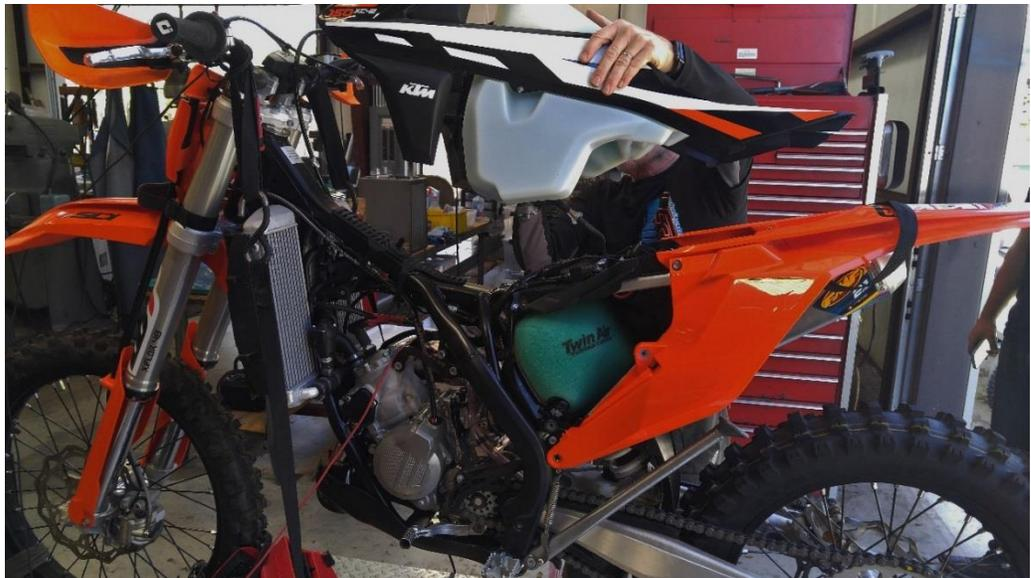
**Step 3:** Loosen the top subframe bolts and remove the silencer or reposition the connecting boot so you can raise your subframe and access your carburetor.
