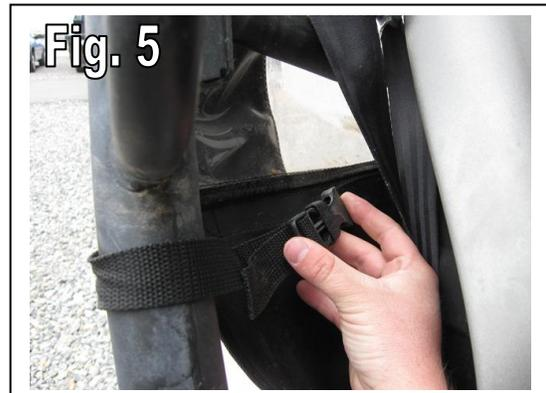
4. Remove the rear seat cushions for easy access to route the bottom straps around the seat mounting frame members. Route the passenger side bottom strap down below the outside seatbelt mounting bracket (fig. 6), across the seat frame members, down under the inside seatbelt mounting bracket (fig. 7) and up to the female buckle located in the bottom middle of the rear window (fig. 8). Repeat this process on the driver side.
