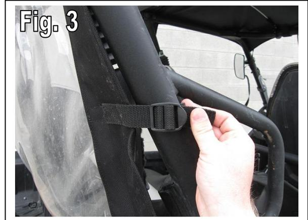
3. Attach the bottom side straps. Loop the straps around the backside of the vertical roll bar, under the bottom of the handhold bar and over to the female buckle (see figs. 4 and 5). Leave straps loose.
