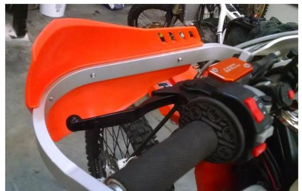
***Caution:*** Check for proper throttle operation after install. Make sure throttle does not stick and rotates freely. Insure that brake and clutch lever have plenty of clearance and don't come in contact with the handguards.
