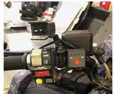
8. Harness may have excess length depending on the application. This can be tied together and hidden in headlight pod or underneath an access cover.
