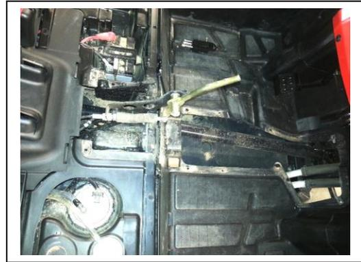
2. Feed harness from the front hood down towards the firewall of the machine. We followed the OEM harness route. Make sure the front of the harness ends up towards the backside of the dash and the rear of the harness at the back of the UTV. Make sure the harness is safe from heat and moving parts of the machine. Do not zip-tie the harness in to place yet.
