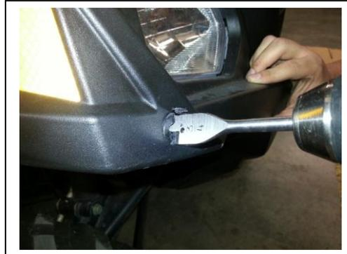
5. To mount the signal, first remove the rubber grommet from the light. Push the grommet into the hole until it is seated correctly into the hole. Feed the wires of the light into the new hole you drilled. Notice the direction on the lens; make sure the "Top" is at the upper point of the light. Plug the black wire from the signal into the positive wire on the harness and the white signal wire into the ground signal wire.
