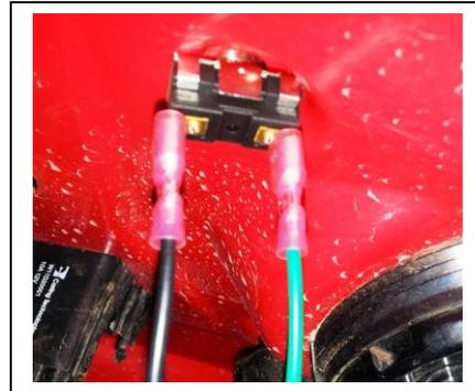
14. To mount the indicator lights, drill a 5/16" hole on both the left and right side of the turn signal switch. Feed the wires of each indicator light through the hole and thread on the nut to secure the light. Plug in the lights, but make sure the indicators are connected to the correct wires on the harness (again, refer to the wire diagram).
