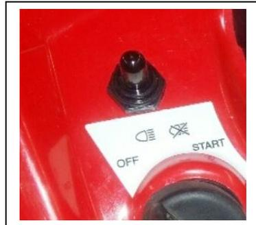
12. To mount the horn switch, drill a 1/2" hole in the desired area in the dash. Install the switch through the hole and put the sealed rubber nut on.
