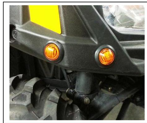
6. Repeat steps 3-5 to install the rear signals for the machine. Remember that the polarity on LED lights is critical. Please refer to the Wire Harness Diagram included with the harness packaging to ensure you get the positive and negative wires correctly in place.
